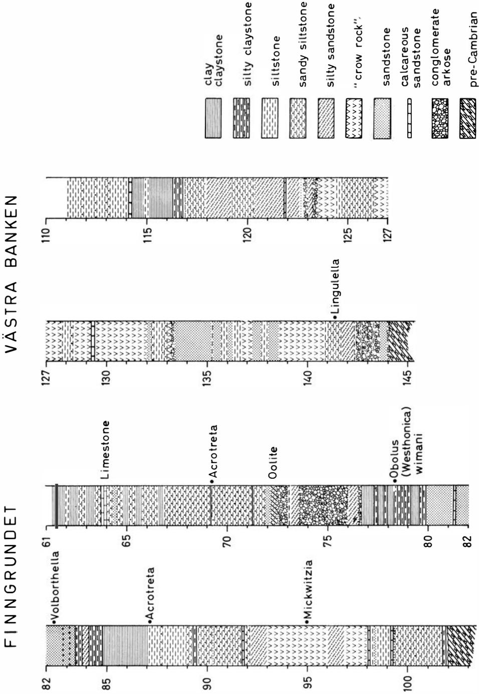
Fig. 4. Diagrammatic sections of the Lower Cambrian strata of the Finngrunden shoals.
