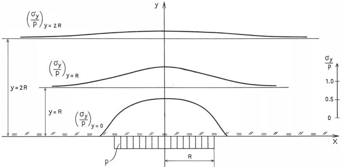
Fig. 8. Normal stress distribution in the centre of an elastic, homogeneous structure loaded perpendicular to
