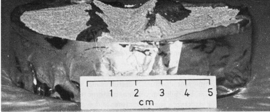
Fig. 53. Two anticline ridges of stitching wax protruded through an overburden of painter's putty with sheet of concrete on the surface.
