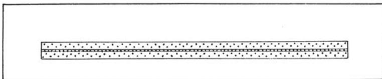
Fig. 28. Cross section through model S 52 prior to run in centrifuge. Dotted: red silicone putty,  $\rho = 1.14 \text{ g/cm}^3$ ; vertical lines: white silicone putty,  $\rho = 1.14 \text{ g/cm}^3$ ; white: painter's putty,  $\rho = 1.87 \text{ g/cm}^3$ .
