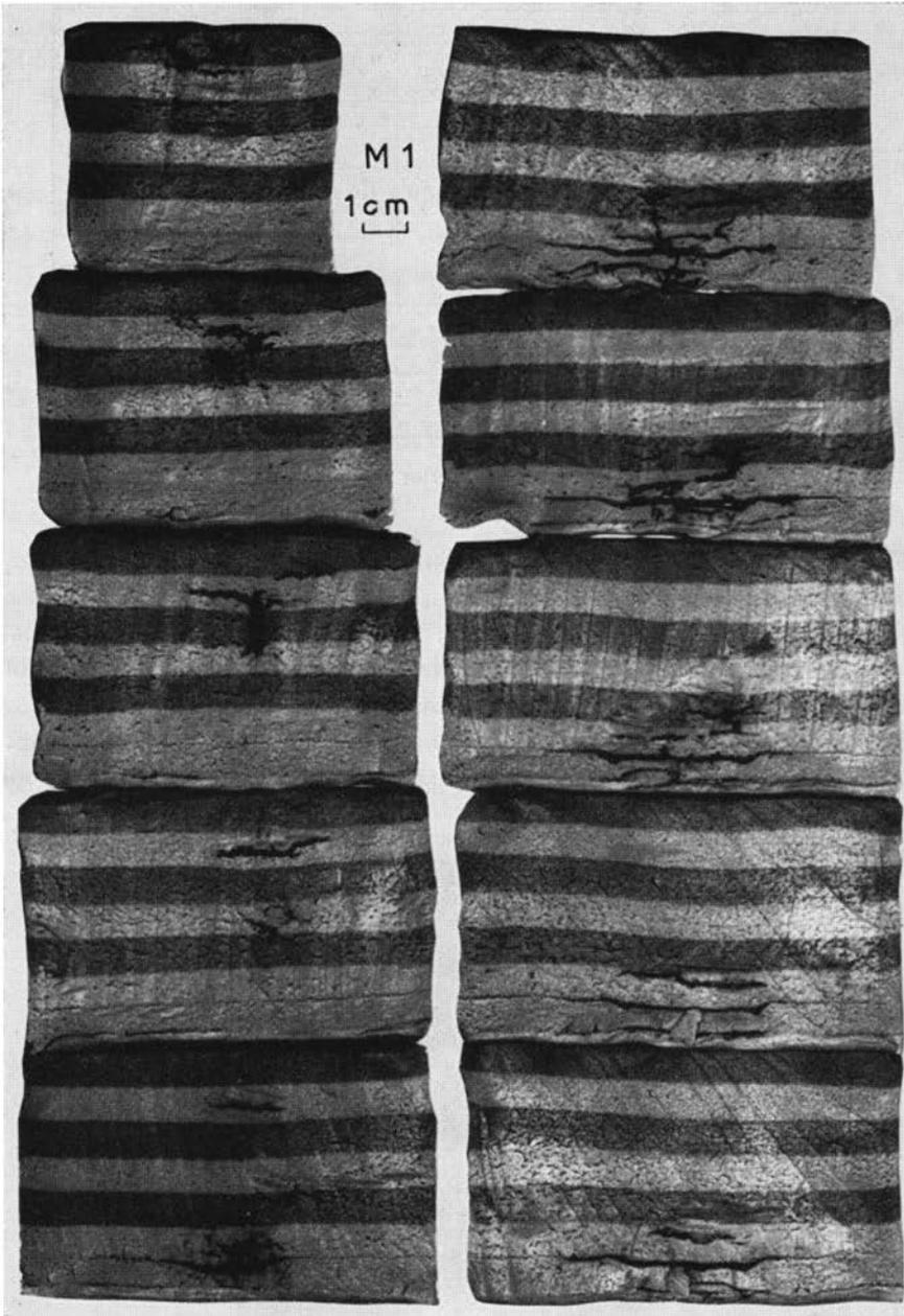
Fig. 3. Sections through a dynamic model (M 1) of a magma-imitation fluid (a  $\text{KMnO}_4$ -solution) rising through the imitation crust (layers of putty with unlike color) as run for 15 minutes at 210g in a centrifuge with the centrifugal force pointing downward in the figure. The dark irregular spots within a central vertical zone of the sections show the uneven path of the rising "melt".
