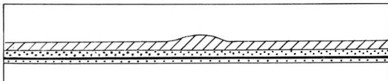
Fig. 20. Model as shown in Fig. 19 prior to run in centrifuge. Dotted with black line: source layer of silicone putty with layer of modelling clay; inclined hatching: oil-wax mixture; white: painter's putty.
