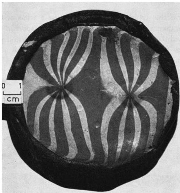
Fig. 38. Deformation of source layer around two domes. The figure shows the under side of a source layer of silicone putty consisting before run of straight strips of alternating light and dark colors. To prevent drag along the bottom the source layer was floating on mercury during run in centrifuge, and the deformation pattern shows how the material was sucked toward the roots of the two domes resulting in an intensive stretching in the region between the domes.
