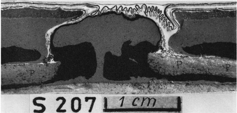
Fig. 70. Cross section through model S 207, which is quite similar to model S 206, showing intensive buckling and stretching of surficial multi-layer in connection with the domal rise of the light silicone and the subsidence of the sheet of heavy painter's putty (P).
