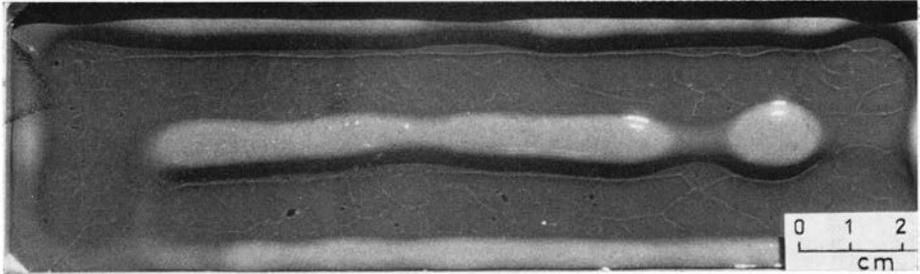
Fig. 11. Anticline of silicone putty, density  $1.14 \text{ g/cm}^3$ , developed due to buoyancy when overlain by heavy syrup.
