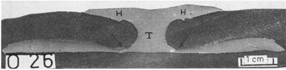
Fig. 13. Cross section of dome of silicone putty (light grey) pierced through overburden of painter's putty (dark grey) with well developed marginal sink (arrows), trunk (T) and hat (H).
