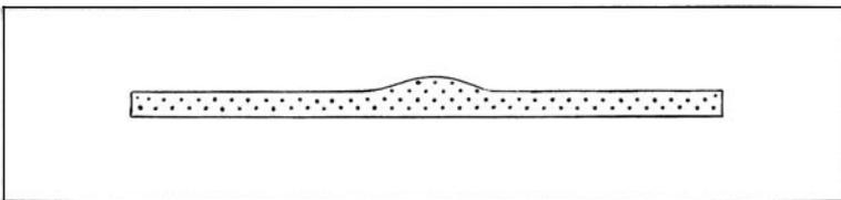
Fig. 14. Model O 26 before run in centrifuge. Dotted: silicone putty; white: painters putty. Bulge on source layer made in order to determine the site of dome formation.
