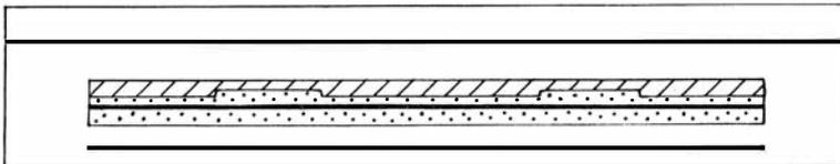
Fig. 18. Section through model S 72 before run. Dotted: silicone putty,  $\rho = 1.14 \text{ g/cm}^3$ ; white: painter's putty,  $\rho = 1.87 \text{ g/cm}^3$ ; black: modelling-clay sheets; inclined hatching: powdered wax soaked in oil,  $\rho = 0.9 \text{ g/cm}^3$ .
