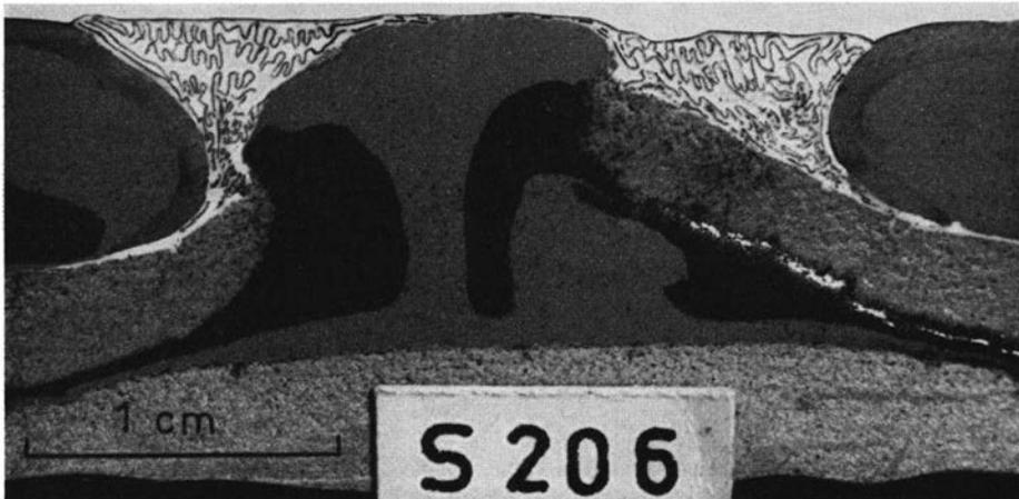
Fig. 69. Enlarged part of model S 206 showing details of buckling structure, the pulling down of the surficial "sediments" in the regions adjacent to the dome, and the boudins formed above the hat of the dome. The boudins are drawn in ink as they may not otherwise show up in the reproduction. See also Figs. 67 and 68.
