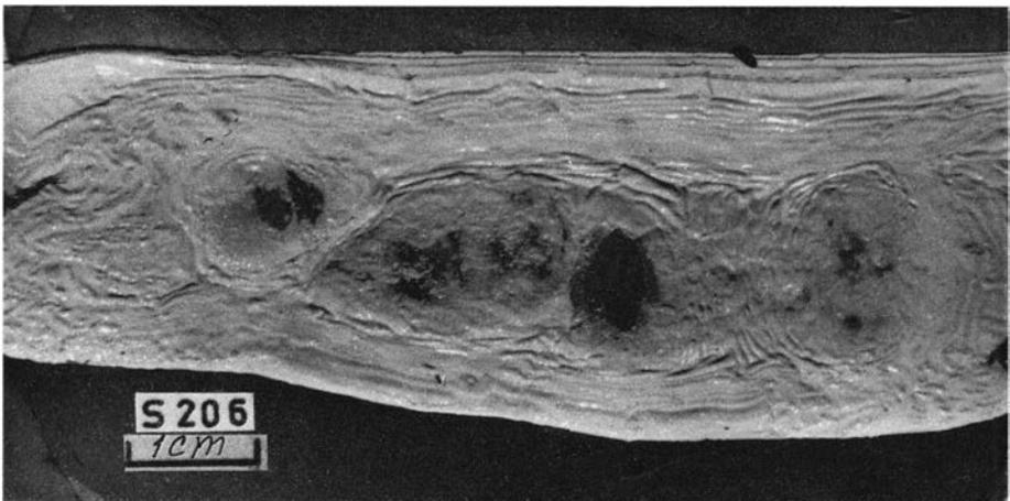
Fig. 71. Model S 206 seen from above after run in centrifuge. Note buckling of surficial layer adjacent to the domes and along the edge of the "geosyncline".
