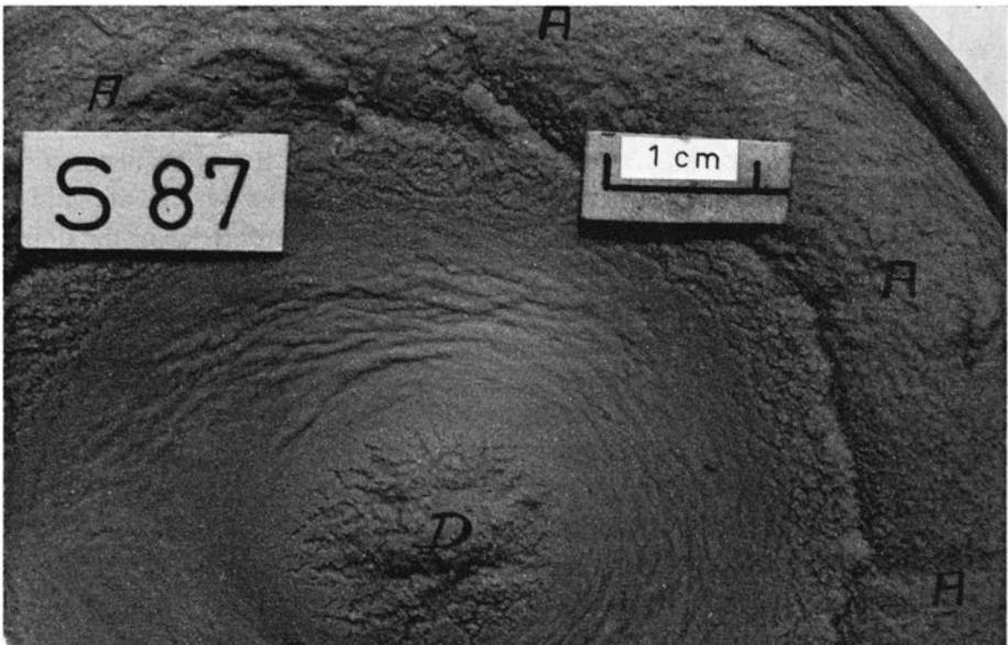
Fig. 34. Buckles of surface of putty overburden in syncline between a central dome (D) and anticline (A) along the edge of the circular model.
