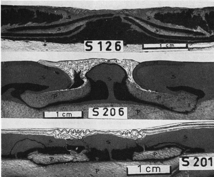
Fig. 68. Sections through models S 126, S 201 and S 206 after run in centrifuge (see Fig. 67). Black layers in S 126: heavy painter's putty. Black massive regions: dark silicone putty; white or light grey with dark lines: silicone putty with sheets of modelling clay; grey, *S*: silicone putty; *M*: sheet of modelling clay; light grey, *P*: painter's putty.
