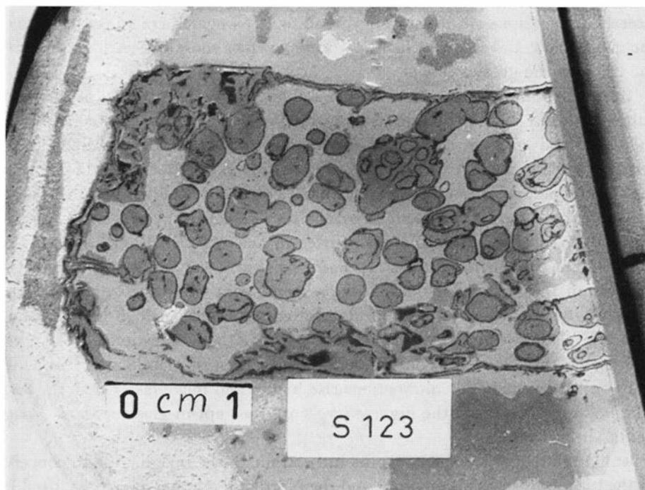
Fig. 51. Model practically identical to S 122 seen from above after run for 10 minutes at 2400g. Dark grey: domes of red silicone putty,  $\rho = 1.14 \text{ g/cm}^3$ ; light grey: overburden of pink silicone,  $\rho = 1.14 \text{ g/cm}^3$ . Dark mantle around domes is remnant of black deep-seated overburden with density  $1.35 \text{ g/cm}^3$ , *i.e.* the buoyancy-generating overburden, see Fig. 50.
