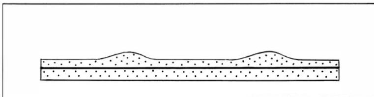
Fig. 30. Cross section of model S 73 before run in centrifuge. Dotted: red silicone putty with thin sheet of modelling clay; white: painter's putty.
