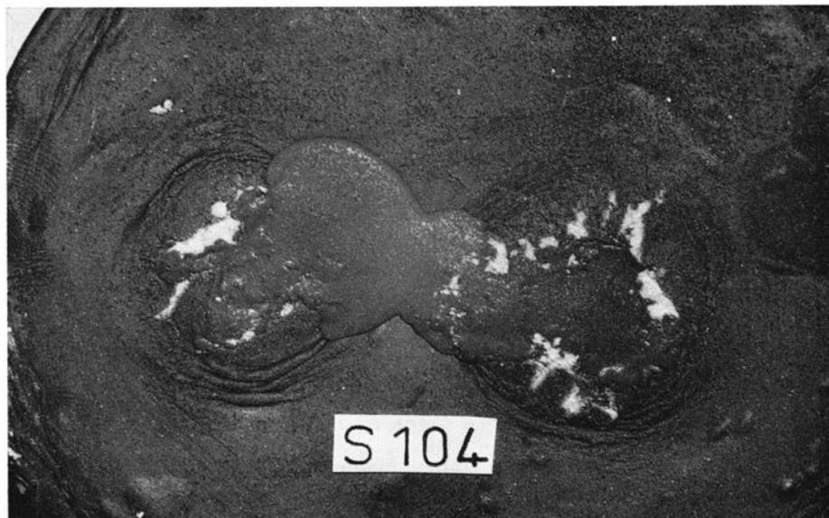
Fig. 35. Buckles and tensional tears in surface sheet of modelling clay above two domes of silicone putty run in centrifuge. Distance between centers of domes about 4 cm.
