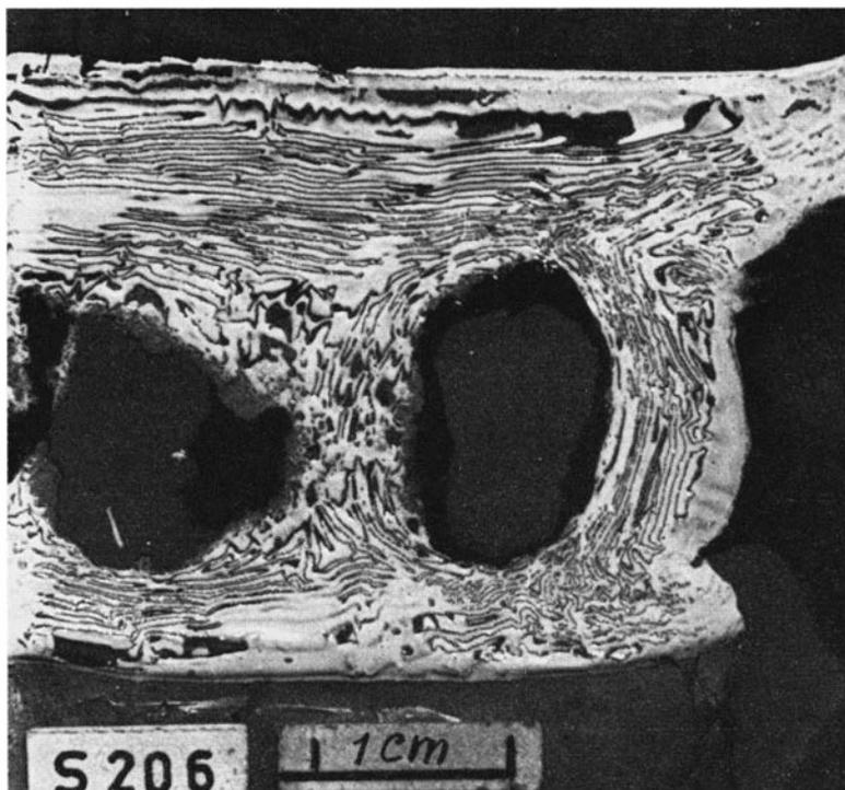
Fig. 72. Model S 206 as seen from above after half of it cut away for sectioning and a thin sheet cut off from the top to show the fold pattern of the surficial multilayer.
