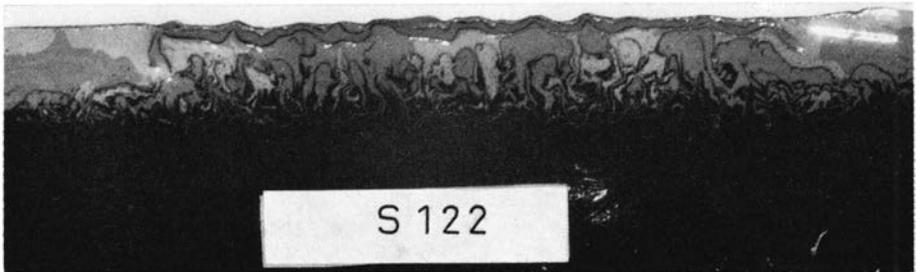
Fig. 49. Domes of silicone putty (light and darker grey),  $\rho = 1.14 \text{ g/cm}^3$ , which have risen through three layers of black silicone putty,  $\rho = 1.35 \text{ g/cm}^3$ , see Fig. 50.
