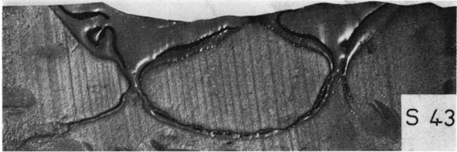
Fig. 36. Model of double-dome of silicone putty with boudins of modelling clay in overburden of painter's putty. Late stage of evolution.
