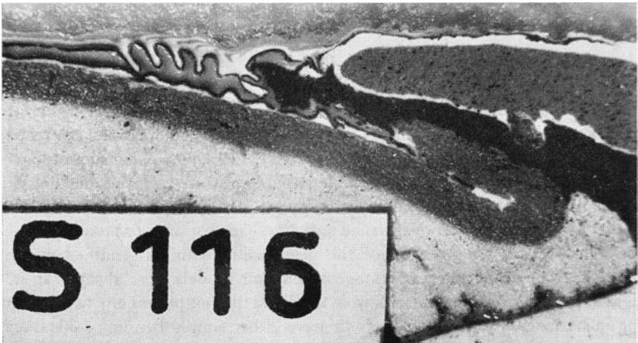
Fig. 62. Enlarged edge of model S 116 showing front of pennine-type nappe with buckling of "sediments" and inversion of layering. Note e.g. detachment folds of upper thin sheet of modelling clay in front of nappe.
