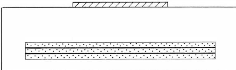
Fig. 46. Model S 48 before run. Dotted: source layer of silicone with sheets of modelling clay embedded; white: painter's putty; inclined hatching: top layer of modelling clay.
