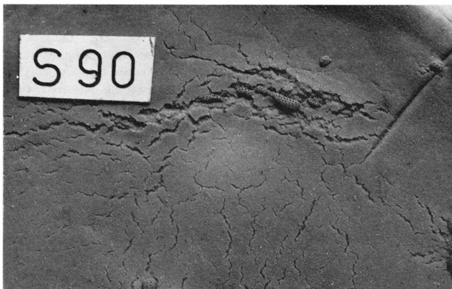
Fig. 48. Tension cracks in overburden of putty through which domes of silicone putty are piercing (dotted). White label about 1.5 cm long.
