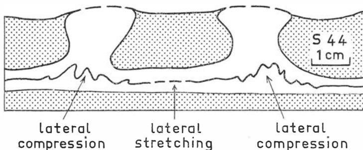
Fig. 42. Cross sections through centrifuged model of double domes of silicone putty (white) with embedded sheet of modelling clay (black) in overburden of painter's putty (dotted). Note intensive buckling of the sheet of modelling clay in the root zone of the domes, and the stretching and fracturing of the sheet in the region between the domes.
