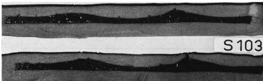
Fig. 16. Cross sections through model showing early stage of dome formation of black silicone putty,  $\rho = 1.34 \text{ g/cm}^3$ , in painter's putty,  $\rho = 1.87 \text{ g/cm}^3$ . Run in centrifuge for 30 minutes at 2000g.
