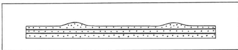
Fig. 41. Cross section of model S 75 before run in centrifuge. Dotted: silicone putty,  $\rho = 1.14 \text{ g/cm}^3$ ; white: painter's putty,  $\rho = 1.87 \text{ g/cm}^3$ ; black: thin sheets of modelling clay.
