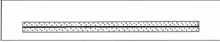
Fig. 26. Model S 93 prior to run in centrifuge. Dotted with black line: source layer of silicone putty with layer of rather stiff modelling clay; white: painter's putty.
