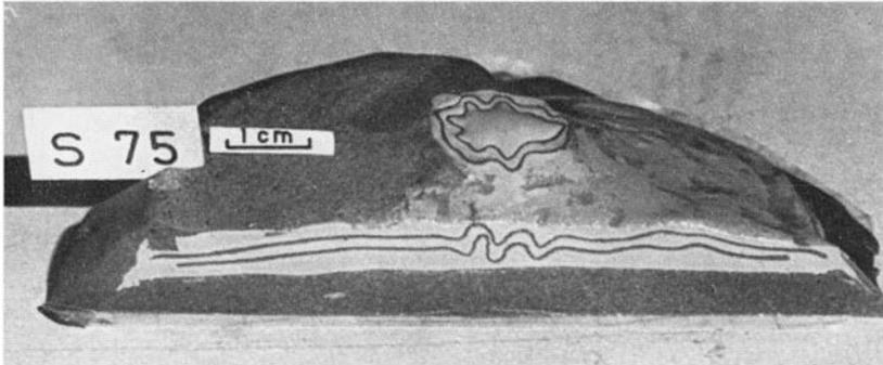
Fig. 40. Model S 75 cut in half after run for 2 minutes at 700g in centrifuge. The photo, which shows one of the two domes formed, shows buckles of the embedded sheets of modelling clay in the region between the domes and in the trunk of the dome which has been cut along a horizontal plane. Part of the overburden has been removed.
