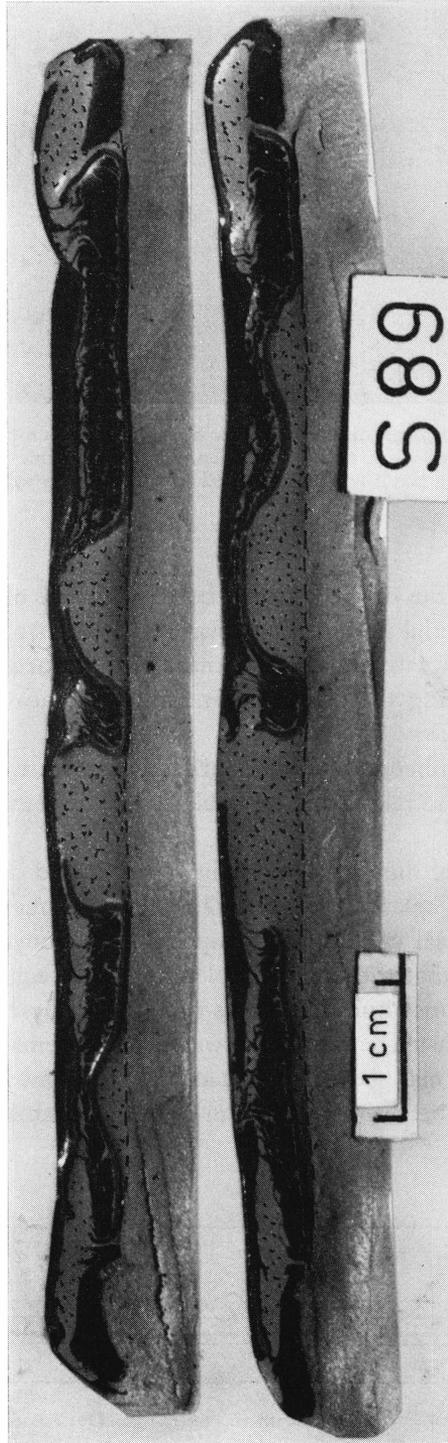
Fig. 21. Sections through centrifuged model of domes of silicone putty (dotted) with density  $1.14 \text{ g/cm}^3$  formed in overburden of heavy silicone putty (dark), density  $1.34 \text{ g/cm}^3$ , with stiff sheet of modelling clay in overburden and in source layer. Light grey uniform substance on bottom is heavy painter's putty. Run for 20 minutes at 2000g.
