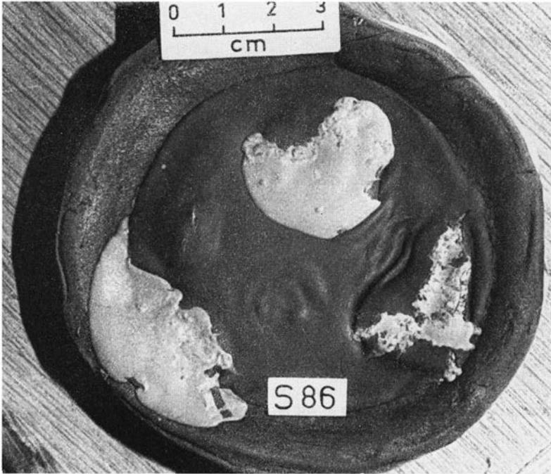
Fig. 33. Model S 86 after run in centrifuge as seen from above. Note pierced domes, tearing of sheet of modelling clay above domes and buckling in front of spreading domes.
