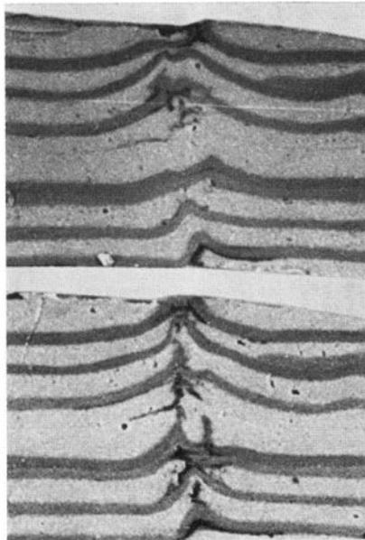
Fig. 5. Cuts through the vent along which a solution of  $\text{KMnO}_4$  has risen through a layered overburden of putty and modelling clay, run in a centrifuge for less than 1 minute at  $1000g$  with the centrifugal force pointing downward in the figure. Height of cuts about 3.5 cm.
