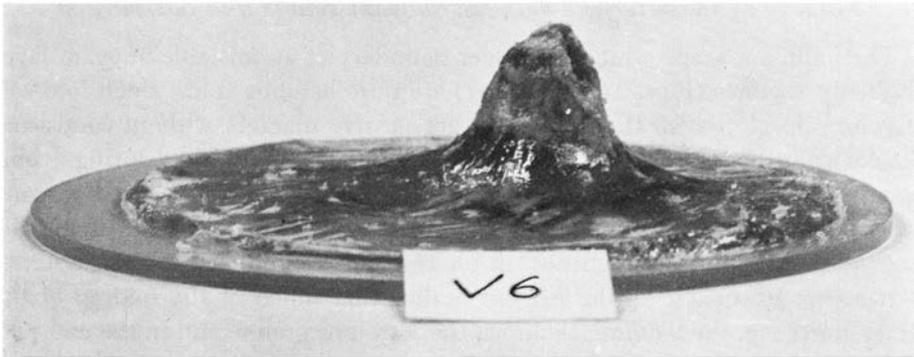
Fig. 23. Stitching-wax dome grown in overburden of putty, run in centrifuge. Overburden removed. Diameter of bottom plate 10 cm.
