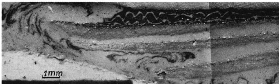
Fig. 47. Buckling of "sedimentary" strata in front of a spreading dome in model S 120. Light uniform grey with dark "sliren": silicone putty; darker grey with granular texture: overburden of painter's putty; black with buckled sheets of white material: dark silicone putty with sheets of modelling clay. The model is similar to S 121, Fig. 65.
