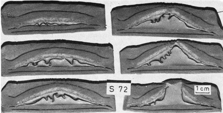
Fig. 17. Sections through centrifuged model of silicone putty, painter's putty, modelling clay and wax powder arranged as shown in Fig. 18 before run. Note the very broad shape of the dome, the buckling of the competent dark sheet in the doming body, and the boudinage of similar sheet in overburden. Run for 10 minutes at 1300g.
