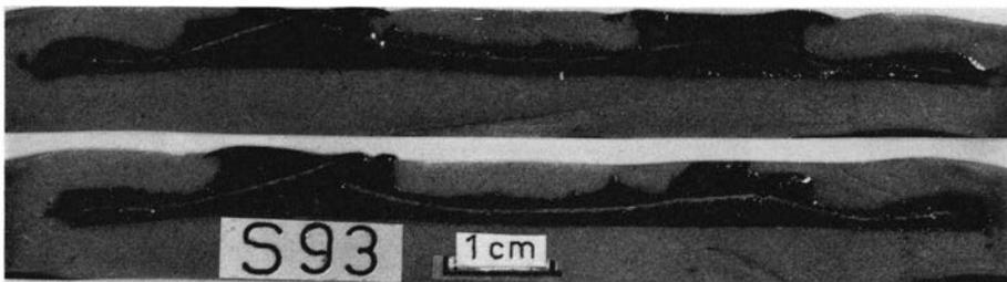
Fig. 25. Cross sections through model with domes of black silicone putty (density  $1.38 \text{ g/cm}^3$ ) with thin sheet of rather stiff modelling clay. Overburden and substratum consist of painter's putty with density  $1.87 \text{ g/cm}^3$ . Run in centrifuge for 15 minutes at 1300g.
