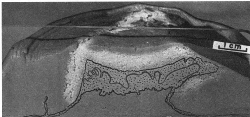
Fig. 19. Section through centrifuged model similar to S 72 but with somewhat thicker layer of powdered wax between source layer and overburden. Dotted: silicone-putty "dome" (note buckled layer of modelling clay); white: oil-soaked wax; uniform grey: painter's putty.
