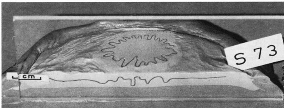
Fig. 29. Model S 73 after run in centrifuge. The model is cut in half, the putty overburden is removed to show the source layer with the buckled sheet of modelling clay, and the dome is cut horizontally about 7 mm below the original surface.
