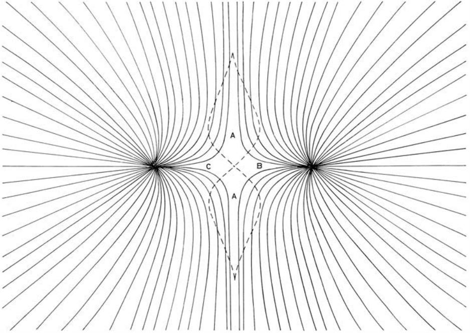
Fig. 39. Flow lines (particle paths) for flow in source layer toward two domes close enough for their flows to interfere, see text.
