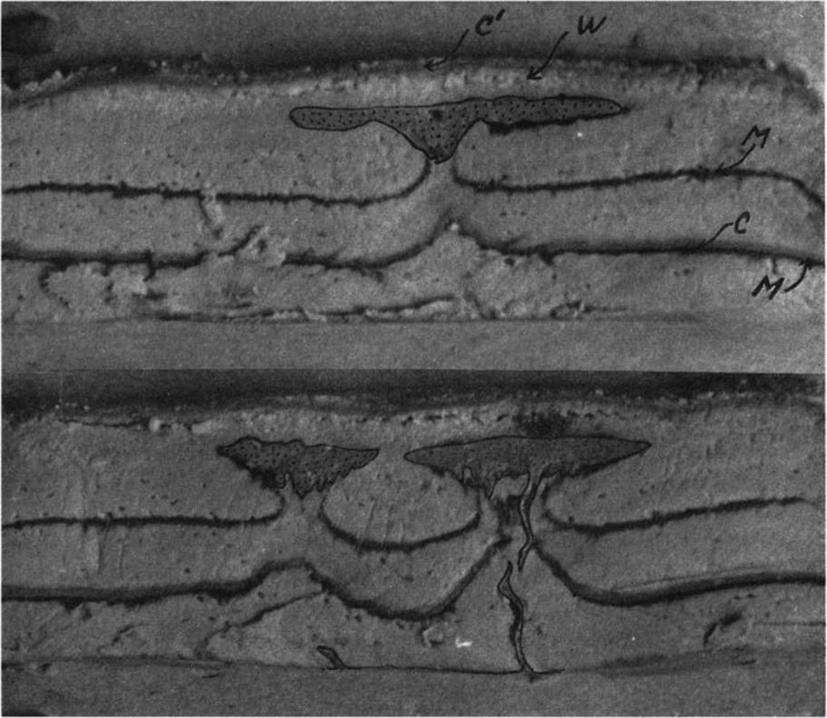
Fig. 64. Model of buoyant body (dotted) which has spread out under a layer with low density (w) (RAMBERG 1963).
