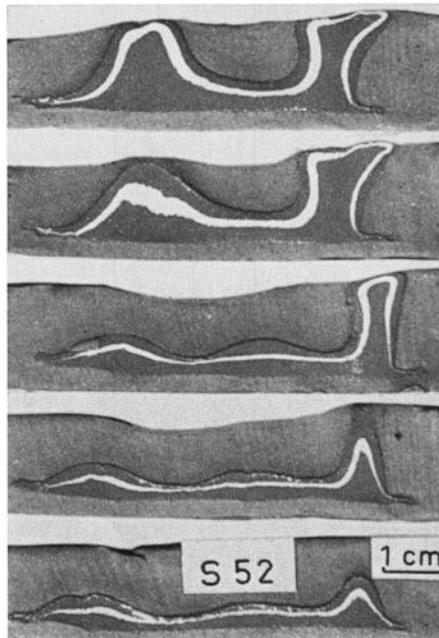
Fig. 27. Cross sections through centrifuged model of domes of silicone putty (grey, with smooth texture) with layer of white silicone putty developed in overburden of painter's putty.
