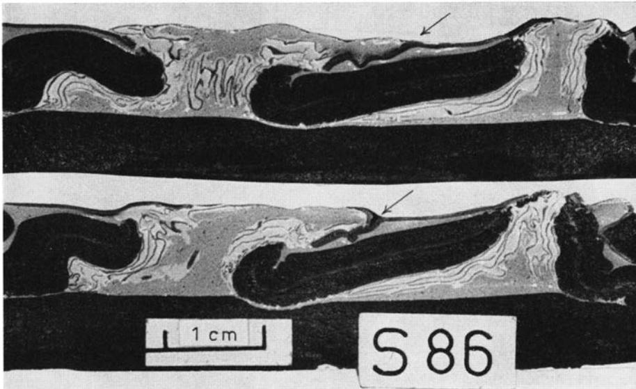
Fig. 31. Cross sections through model of silicone domes with thin sheets of modelling clay and overburden of painter's putty (black) after run in centrifuge for 15 minutes at 1300g. Note recumbent folds at arrows.
