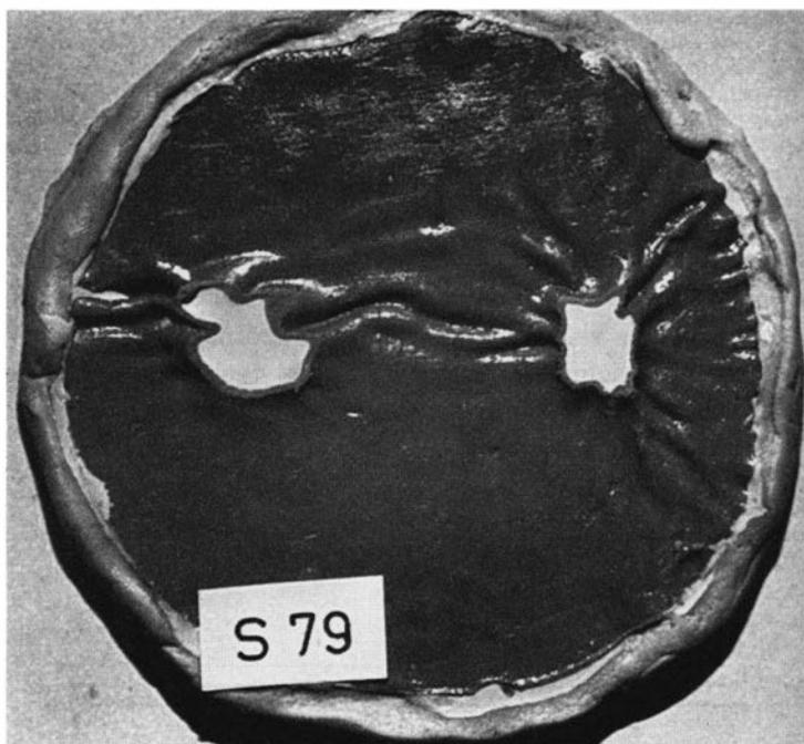
Fig. 44. Centrifuged model of two domes of silicone putty (white) with thin top sheet of modelling clay (dark grey) rising through an overburden of painter's putty (removed in photo). Note buckling of modelling-clay sheet around and between domes.
