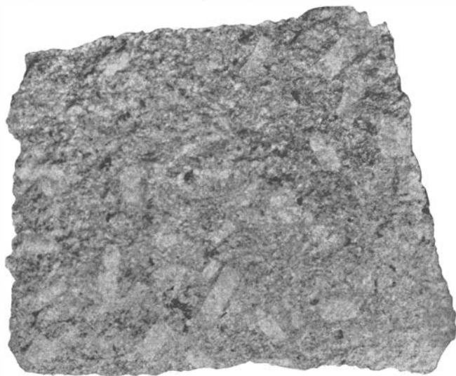
Fig. 36. Analcitised aegirine-augite-syenite porphyry (1:1), No. VI, Sample 301, from Liang Chia P'o.
