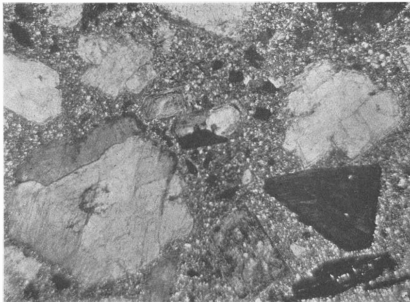
Fig. 28. Banatite porphyry ( \times 13 , Nic. +) from Lung Wang Miao intrusive.
