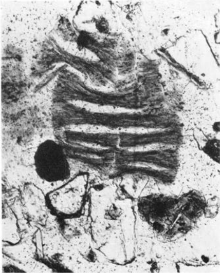
Fig. 6. Crystal of illitic mica with intercalations of the groundmass. 205.26: 3. 110 \times .
