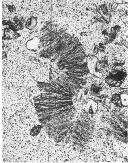
Fig. 5. Vermicular crystal of illitic mica. 205.13: 3. 110 \times .
