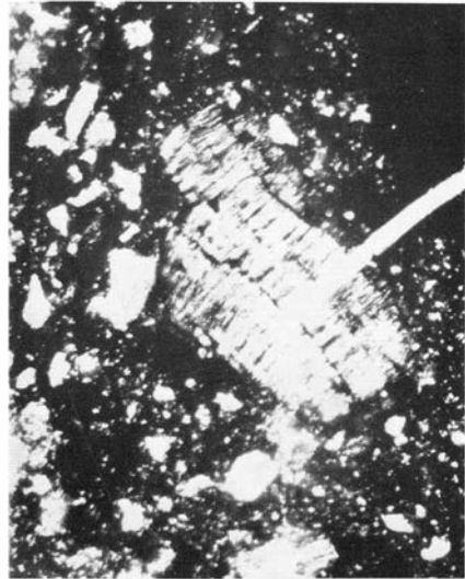
Fig. 7. Crystal of illitic mica with basal cleavage and transverse parting. 205.10: 3. 110 \times 2 nic.
