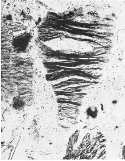
Fig. 4. Part of concretionary aggregate of illitic mica. 205.25: 1. 110 \times .
