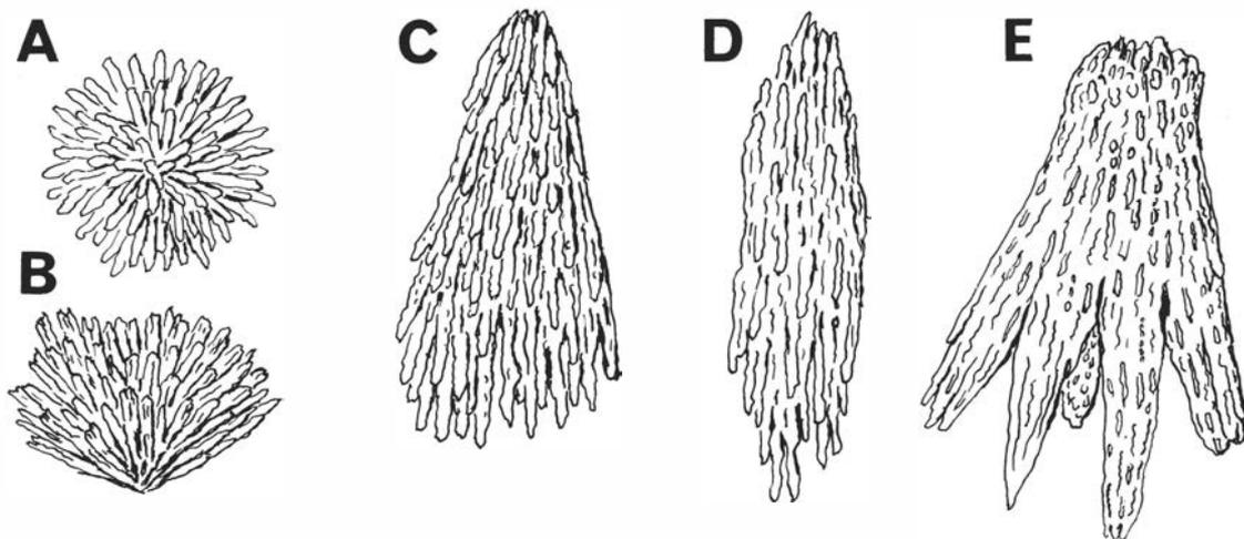
Fig. 1. Structural relationship between spherulites and prisms. *A*, spherulite with regular spherical orientation of the crystallites; *B*, incomplete spherulite with crystallites developed only in the upper half; *C*, prism composed
