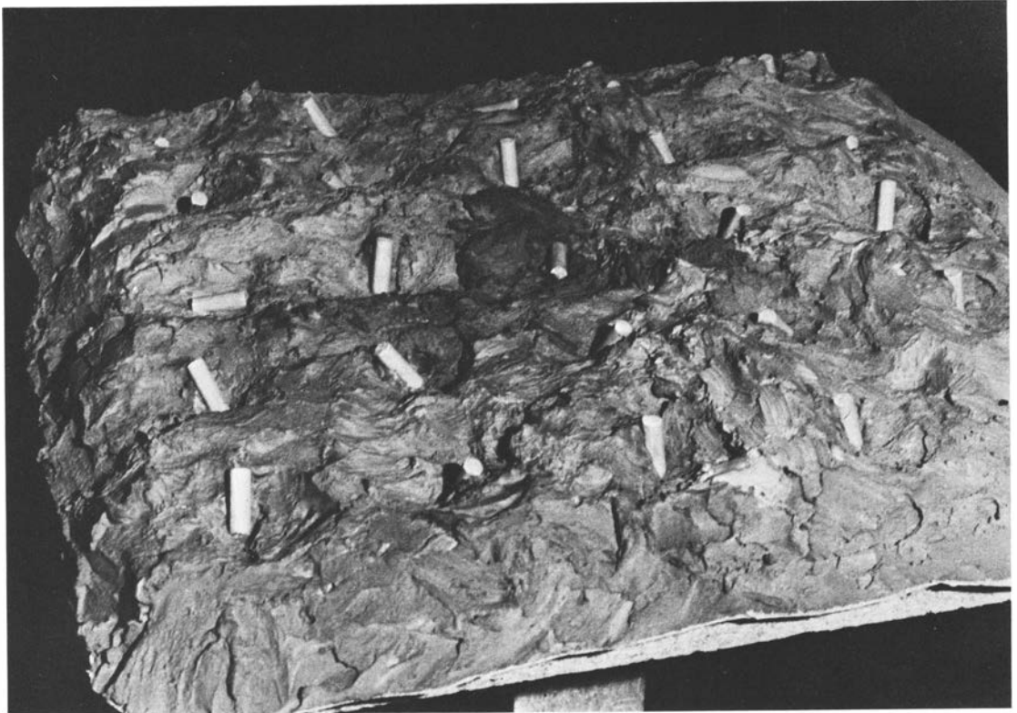
Fig. 1. Artificial till fabric representing pebbles with an a:b axis ratio of 6:2.
