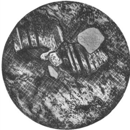
Fig. 5. Inclusions of albite (striped) in microcline.
