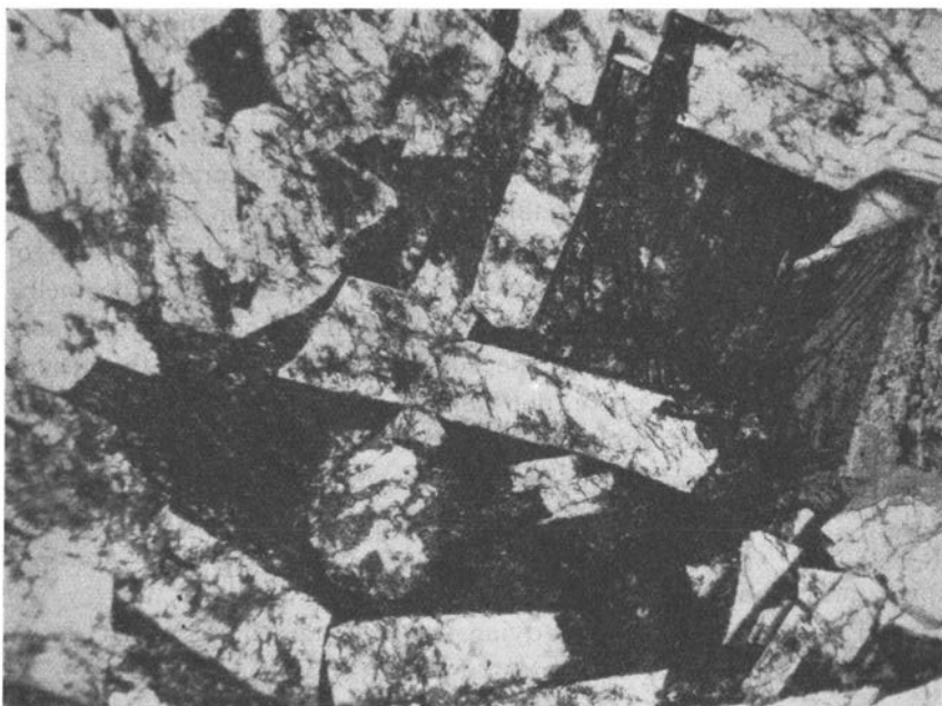
Fig. 6. Microphotograph of the glassy marginal dolerite showing plagioclase laths embedded in a partly devitrified mesostasis. Specimen 236, one nicol. Magnification 40 diameters.
