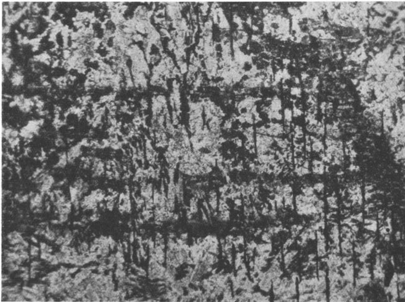
Fig. 20. Groups of fine iron-ore rods perpendicular to long bars of diabantite. Specimen 303, one nicol. Magnification 40 diameters.
