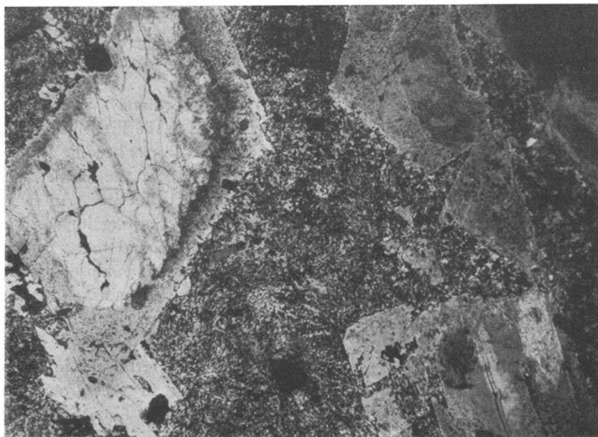
Fig. 23. Idiomorphic andesine phenocryst with an outer albitized border which is irregularly bounded inwards. Specimen 70 a, nicols +. Magnification 7 diameters.
