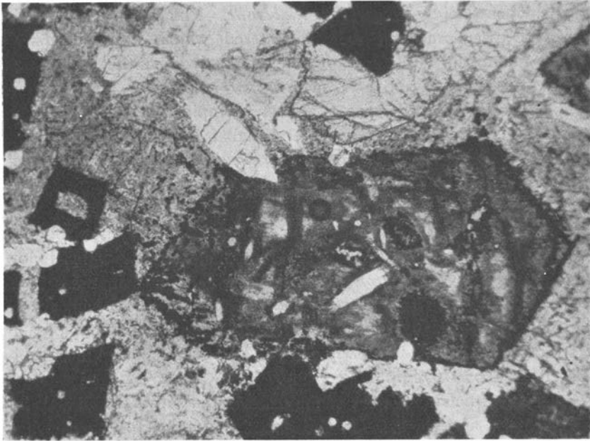
Fig. 13. Idiomorphic olivine pseudomorph in Hällefors dolerite. White inclusion=apatite. Specimen 137, one nicol. Magnification 40 diameters.
