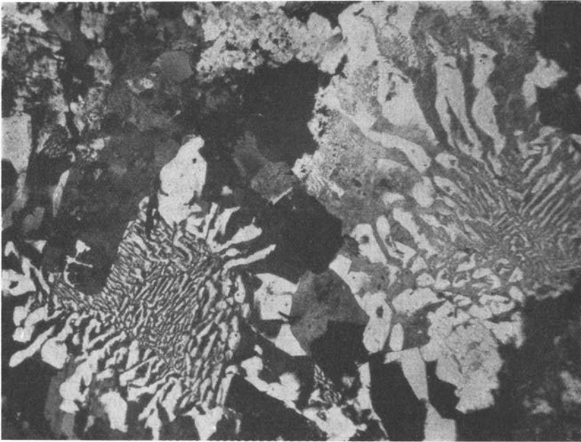
Fig. 5. Micropegmatites in a granitic inclusion in the marginal dolerite. Specimen 148 c, nicols +. Magnification 40 diameters.
