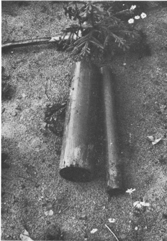
Fig. 1. The measuring tubes used for the infiltration tests. Photograph by T. Olsson.
