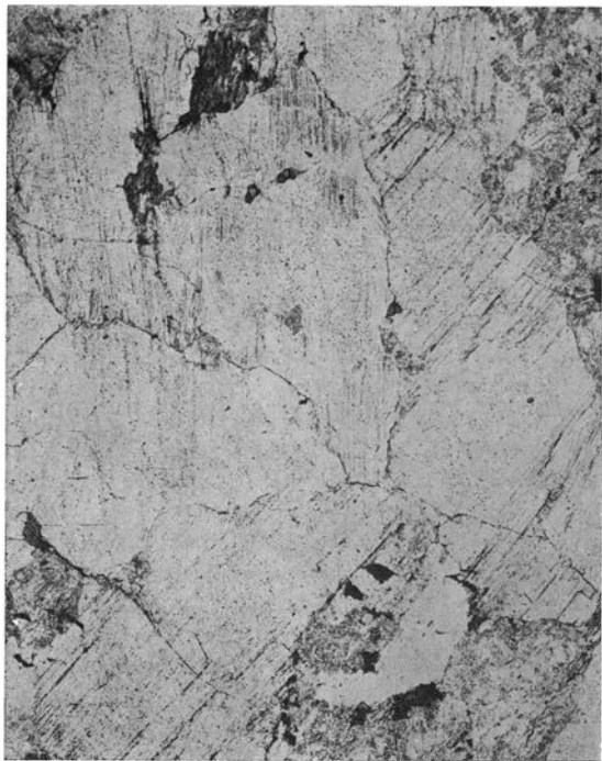
Fig. 3. Granite showing planar elements in quartz. 20 \times .
