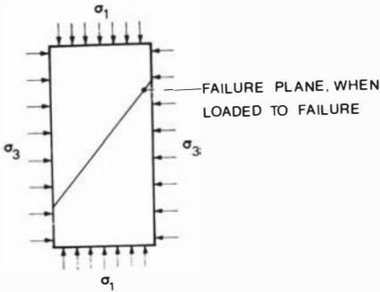
Fig. 2. Specimen under tri-axial compression.
