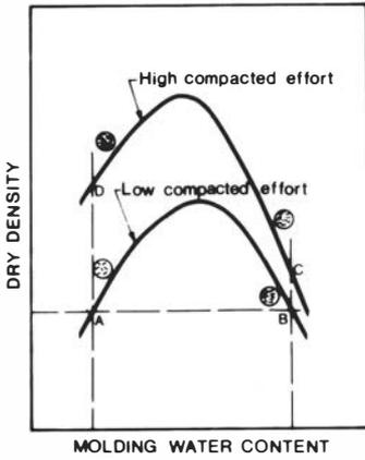
Fig. 9. Effects of compaction on structure (Lambe, 1958).
