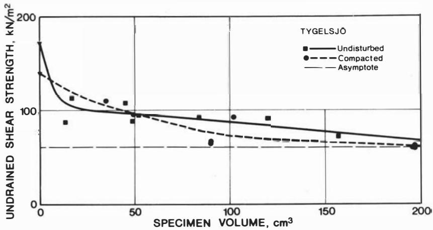
Fig. 6. Undrained shear strength versus specimen volume. Moraine clay from Tygelsjö.
