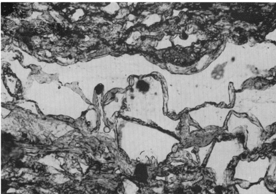
Pl. II, Fig. 2. Detrital ore grain capping a quartz column that penetrates strongly corroded quartz grains (left centre). Plane-polarized light, \times 132 .
