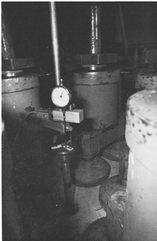
Fig. 4. Close-up of the measuring rod, with strain gauge and a dial gauge. Photograph by A. Carlsson.
