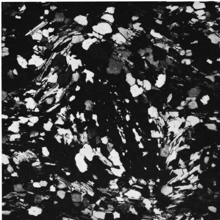
Fig. 5. Elongate garnet relict in quartz argillite schist. Garnet replaced by Fe and Al hydroxides while linear trains of quartz inclusions remain in place. Ba 134, 2 nic., \times 18.5 .
